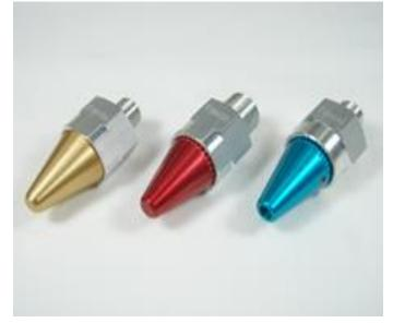
Compressed air flows out along the cone on the outer surface at the speed of sound from the gap around the nozzle circumference. It draws in external secondary air and amplifies it to about 20 times air volume.
